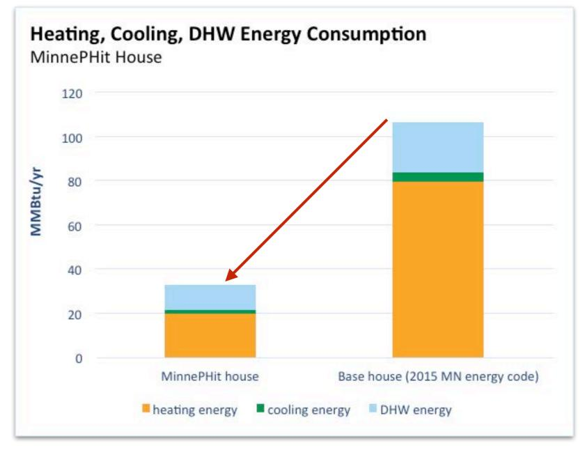
Heat loss is dramatically reduced by more than 66% over current new construction in Minnesota.
