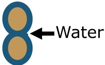
The thickness of these layers increases with increasing water content. At a certain  $X_w$  liquid rings start to form around the contact points between the grains; they show a curved air-water interface.
