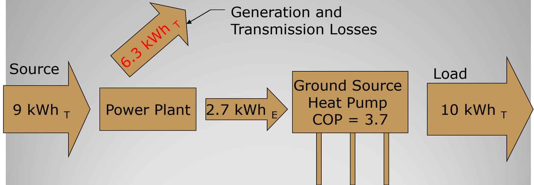
**GSHP requires only  $9 \text{ kWh}_T$  from the source to provide  $10 \text{ kWh}_T$  to the building since they can provide a COP of 3.7**
