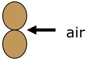
At complete dryness the heat flow passes mainly through the grains, but has to bridge the air-filled gaps between the grains around their contact points.
