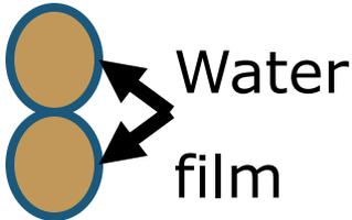
At very low water contents the soil particles are covered by thin absorbed water layers
