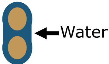
From this point on the thermal conductivity increases rapidly with increasing  $X_w$ , until the rings almost completely fill the original gap. When  $X_w$  increases still further the complete pores are filled with water, up to saturation. This is reflected by the slower increase of  $k$  with  $X_w$ .
